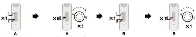
Press the UP and DOWN buttons of remote A simultaneously.
