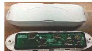
Lift outer cover from circuit board
