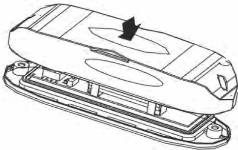
Place the cover over the mounting plate and click into place with a small sideways push.
