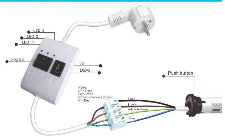
NOTE: When UP/DOWN/PROGRAM button is pressed, light LED1 is on. When PROGRAM button is pressed for 2s, light LED2 is on. When PROGRAM button is pressed for 10s, light LED2 is off and LED3 is on.
