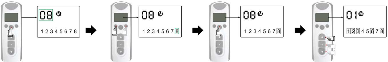
Long press K2 for 2s to enter Group Control mode, the current channel on the upper left corner of the screen will shine.
