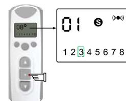
The figure on upper left corner of the screen shows the current channel. Short press K1/K3 to choose any channel from 1 to 8.
