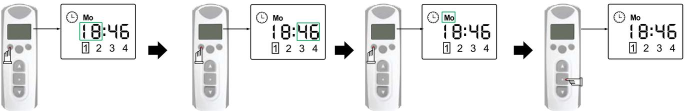
Press K1 button to enter hour setting page, now the hour figure will shine. Press UP/DOWN button to adjust the hour figure.
