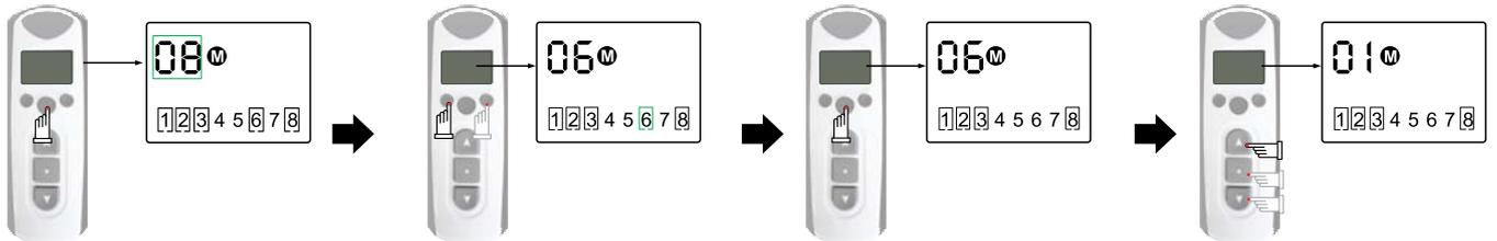
Long press K2 for 2s to enter Group Control mode, the current channel on the upper left corner of the screen will shine.
