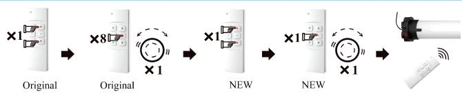
Press the UP and DOWN buttons simultaneously, then release.
