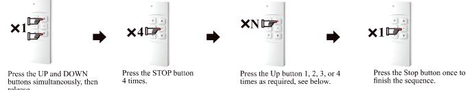
The number of times the UP button (N) is pressed will determine the level of torque applied before the motor will stop at the inner limit. Press once for 25%, twice for 50%, three times for 75% or four times for 100% torque required to stop. (Default is 25%)
